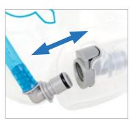
2. To reconnect the hydration tube, simply press the Quick-Disconnect connector back into the port on the reservoir, pressing firmly until the Quick-Disconnect button reengages with an audible "click" and the connector cannot be pushed into the port any further.
